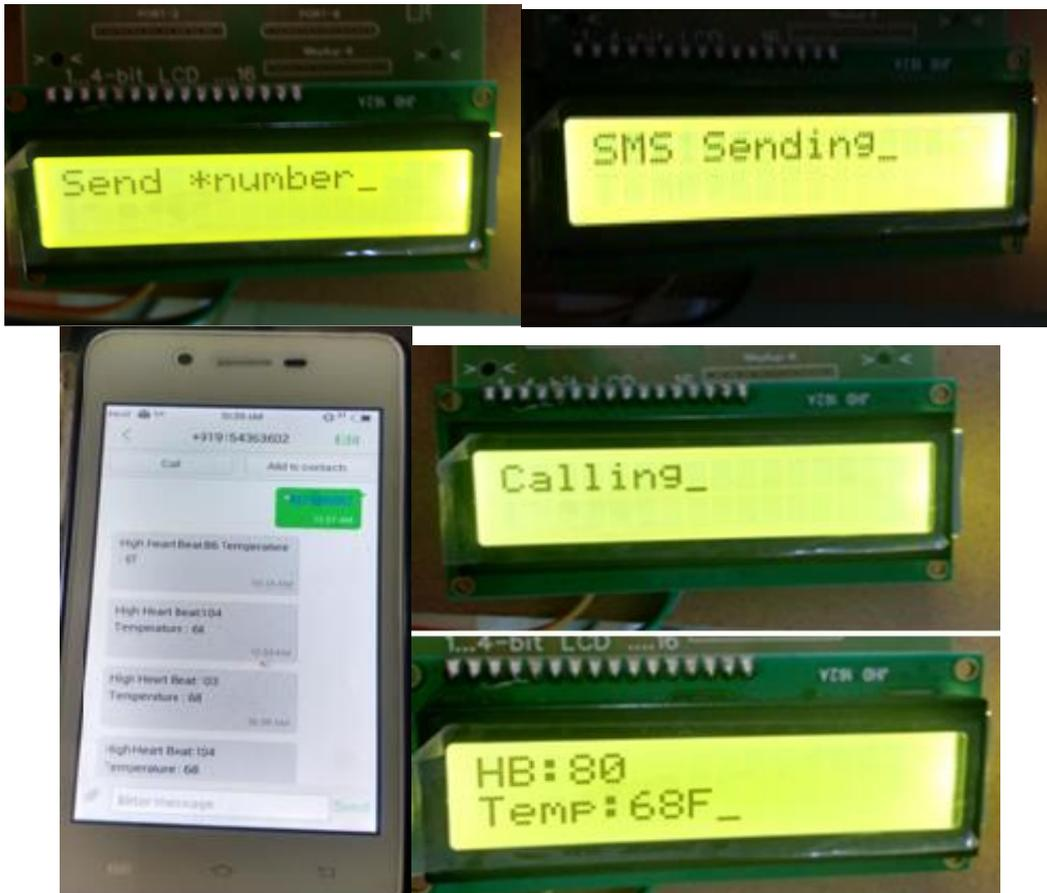
Figure 2: Heart beat and temperature values display and sending to mobile
